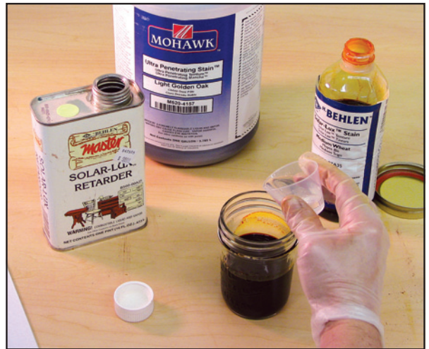
Figure 4.16. Mix one part retarder with ten parts non-grain-raising stain to slow it down enough for hand application.
