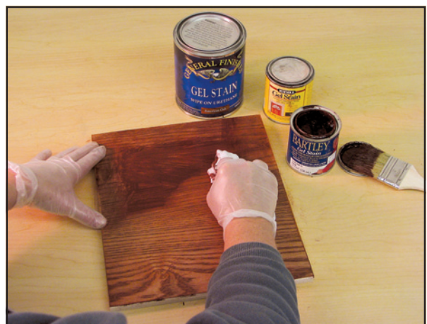
Figure 4.9. Gel stains spread easily with either brush or rag. Work the surface until it has neither streaks nor heavy spots.
