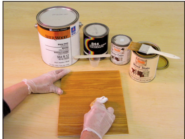
Figure 4.5. Wipe off any excess cleanly. You can adjust the color of quick-dry wiping stains with up to 20% of Chroma-Chem 844 Colorants or Behlen Master Color.
