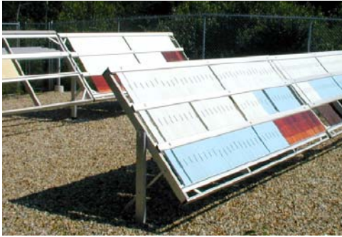
3 Year Exterior Exposure Exterior 450 Base Resin Florida 45° South Exposure
